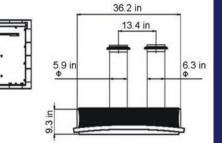
Note: The external pipes have two different diameters, use 6.3 in for inlet side and 5.9 in for outlet side.
