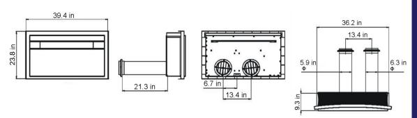
Note: The external pipes have two different diameters, use 6.3 in for inlet side and 5.9 in for outlet side.
