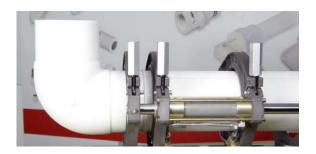
This heat fusion technique involves the joining of plain-end pipe with plain-end fittings, and is suitable for pipe and fittings ranging from 6" and larger. The pipe and fittings are heated while being pressed against a "heated plate" for a specified period of time. The piping is then welded together and cooled (see heat soak times charts in Manual).
